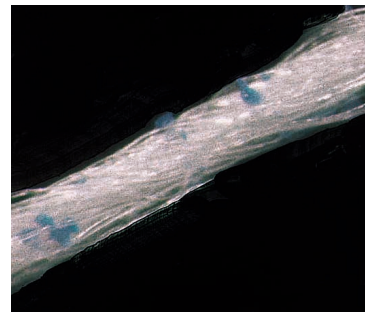
Yarn wax application is particularly effective with an even application.
